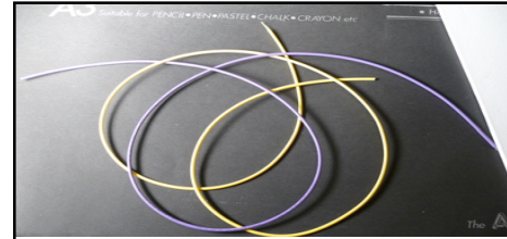
Shrink Tubing. You can slip this over wires to insulate them. Heat with a blow dryer and it will shrink tight.
